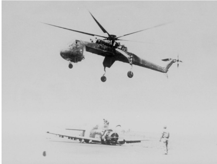
A United States Army CH-54 Flying Crane from An Khe, RVN, brings a crashed A-1 Skyraider from Buoang Briang, RVN to the 633D Consolidated Aircraft Maintenance Squadron for repair. (633 ABW/HO Archive).
