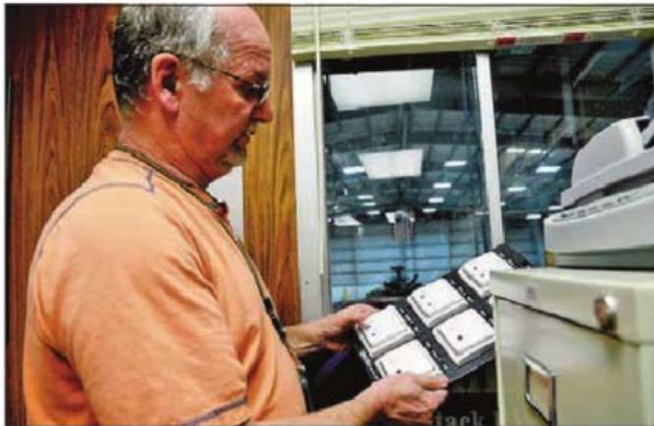
David Malpass, 733rd Civil Engineer Division assistant energy manager, demonstrates how T-5 lights are controlled by a battery-less, wireless control panel at Fort Eustis, Nov. 18. The control panel turns off or dims lighting when not in use, saving energy and money.
