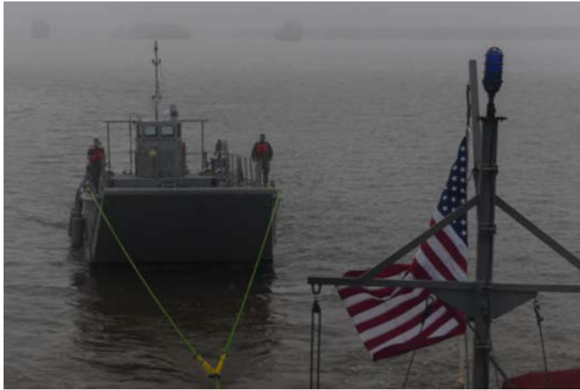
A Landing Craft Mechanized, Mark-8 towed in the Chesapeake Bay during towing training at Joint Base Langley-Eustis, Virginia, 5 Nov 2018. The Small Tug is capable of towing up to 37,000 pounds, which includes a variety in size of vessels to support the installation and brigade objectives. (USAF photo: SrA Derek Seifert).
