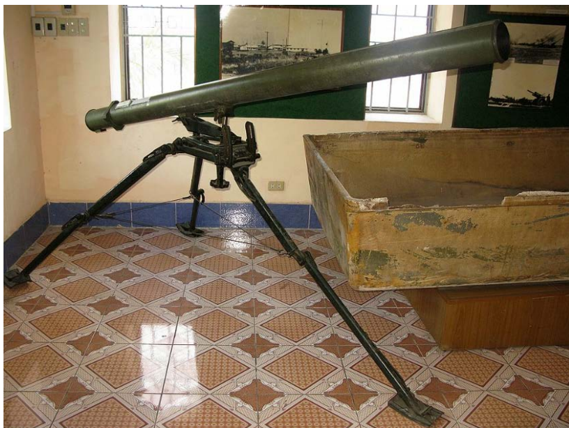
A DKB rocket launcher of the Vietnam People's Army. Grad-P Light portable rocket system. The complete system comprises a single-round man-portable launcher (reloadable), a 122-millimeter high-explosive fragmentation rocket and a fire control panel. The system was developed in the middle of the 1960s for Soviet special units and was used by Vietnamese forces at war with the United States, under the designation DKZ-B. (Photo: Binh Giang, Wikimedia Commons).
