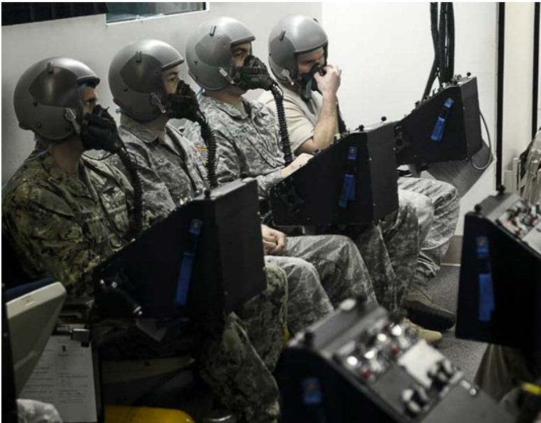
Service members train to recognize and mitigate symptoms of hypoxia in the hypobaric chamber at Langley Air Force Base, 11 December 2014. The hypobaric chamber changes air pressure and chemistry to simulate different heights in altitude to train pilots and aircrew members to handle the physiological stresses of fights. (USAF Photo:A1C Devin Scott Michaels), Cropped).
